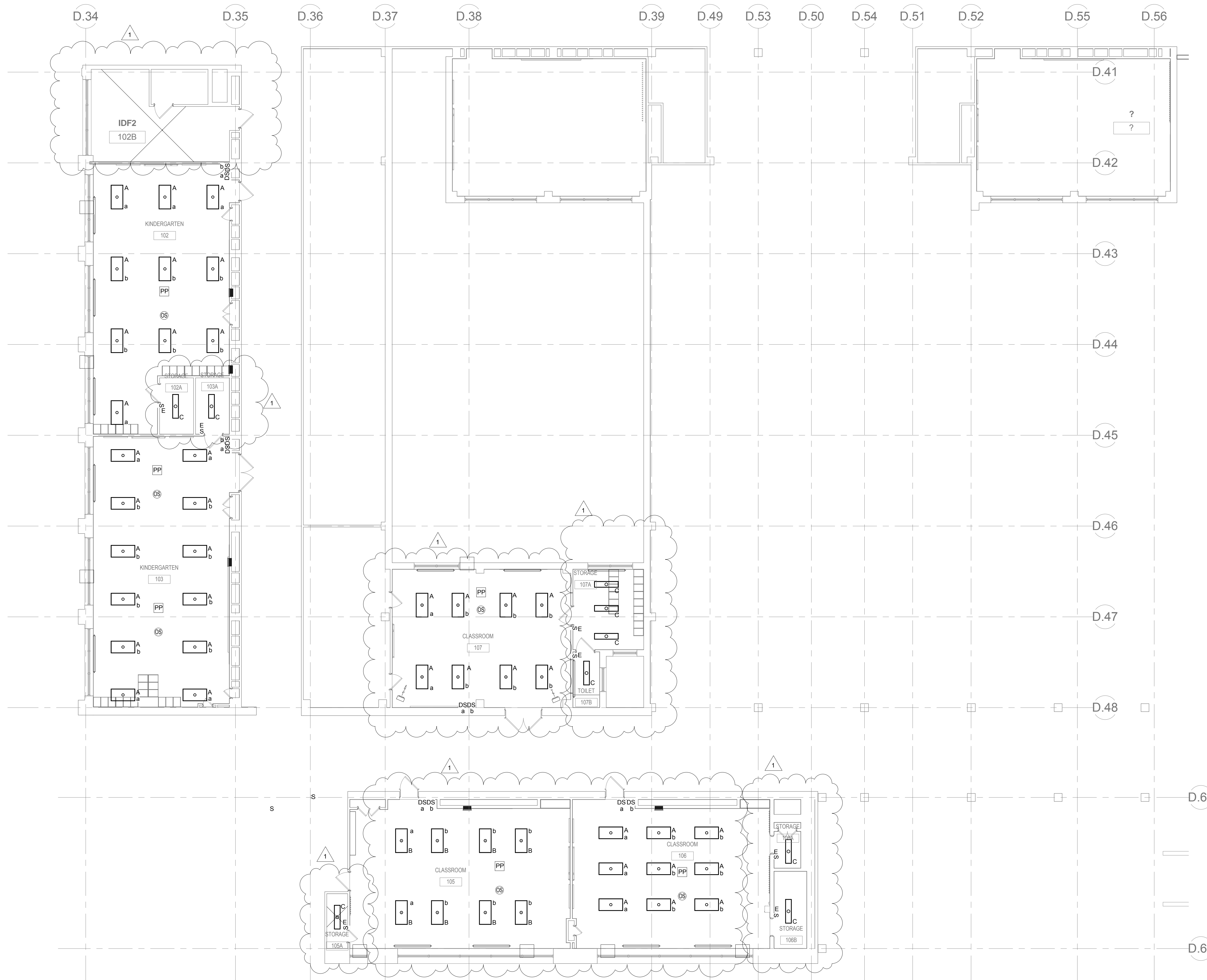
1 FIRST LEVEL - LIGHTING FLOOR PLAN - NEW WORK ROOMS 102, 103, 105, 106, 107, 118 AND 121 1/8" = 1'-0"
