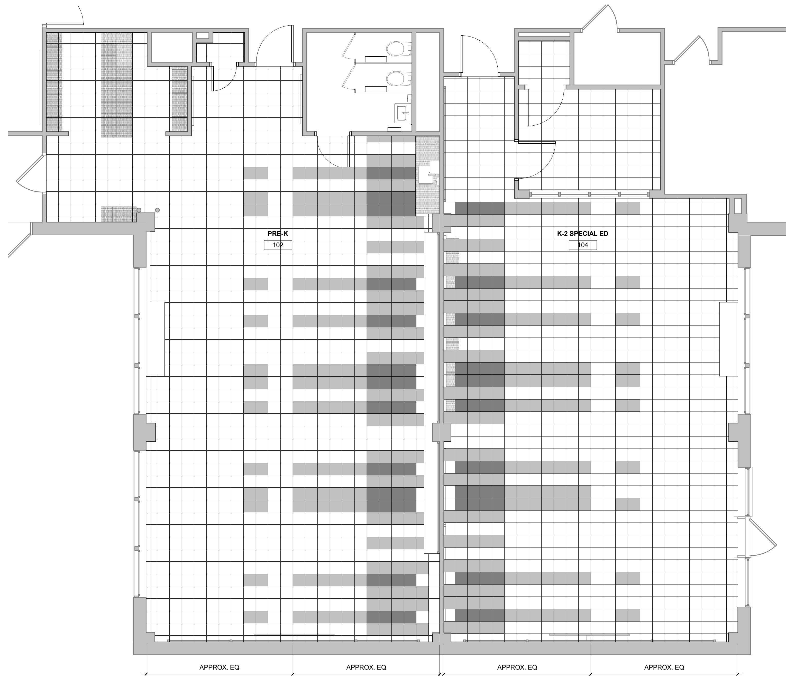
2 ENLARGED FINISH PLAN - FLOOR PATTERN CLASSROOMS 102 & 104 1/4" = 1'-0"
