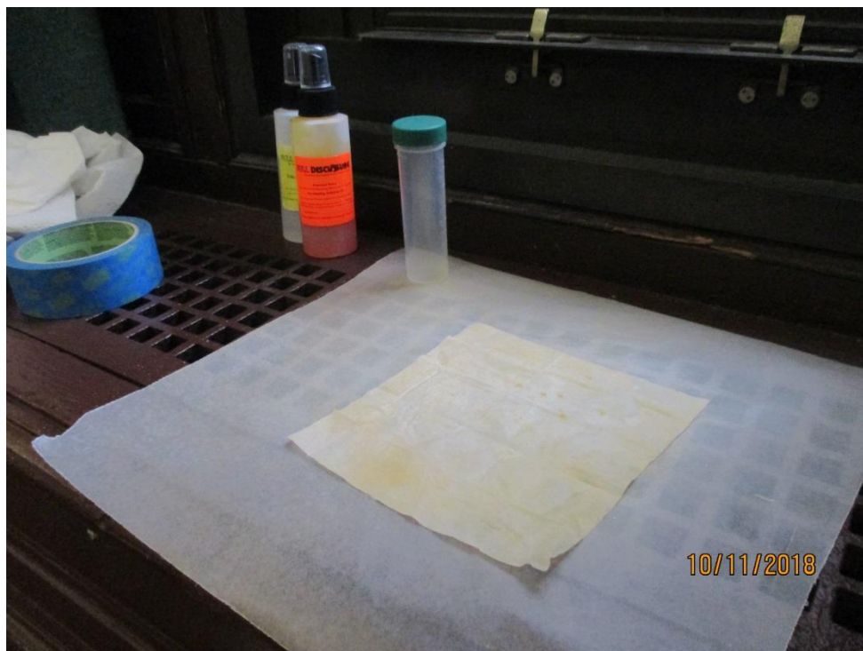
Photo 29 – Colorimetric/Flame AAS Wipe Sample.
