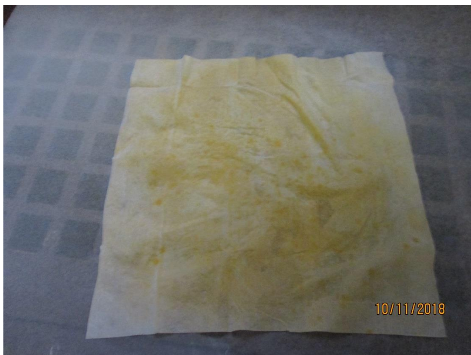
Photo 30 – Colorimetric Wipe Sample (Yellow Color = Passed).
