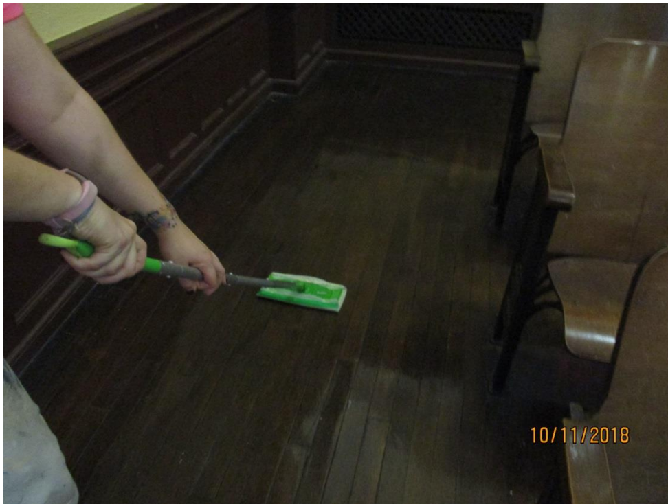
Photo 25 – Swiffer Wipe Testing on a Wood Floor.
