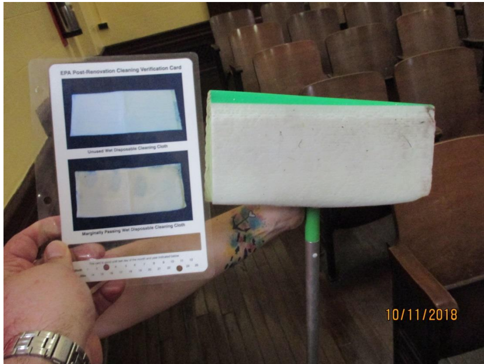
Photo 27 – Passed Swiffer Wipe (per 40 SF) Compared to the EPA Post-Renovation Cleaning Verification Card.
