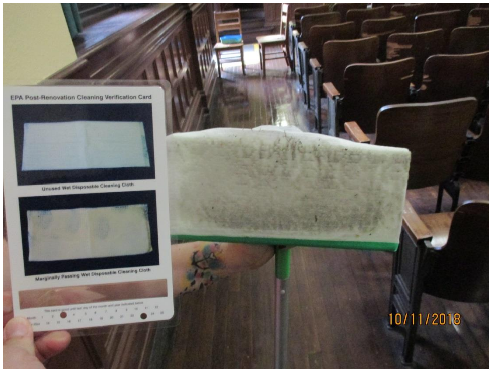
Photo 26 – Failed Swiffer Wipe (per 40 SF) Compared to the EPA Post-Renovation Cleaning Verification Card.
