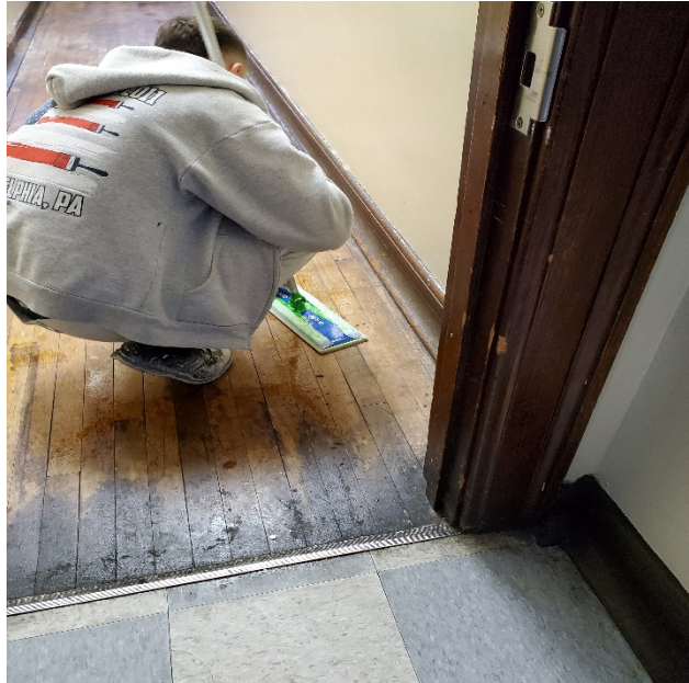
Photograph 5 – RRP wipe on wood floor
