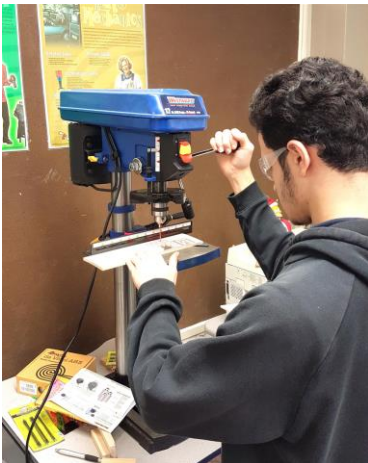
Leandro using drill press to create access holes for scroll saw
